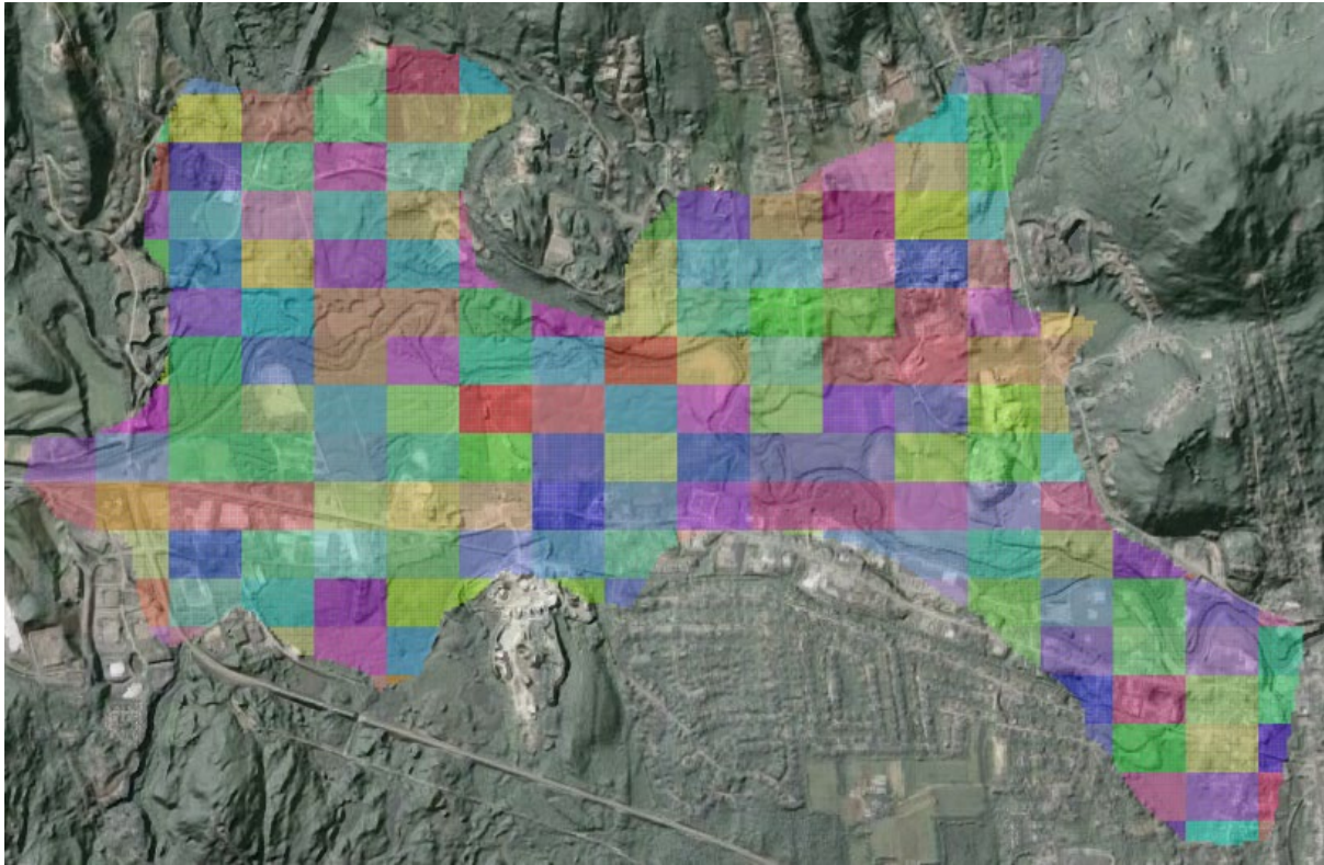
Figure 4.3. Patchwork of drain “reaches”. Observed DRN outflow through each reach is zero.
