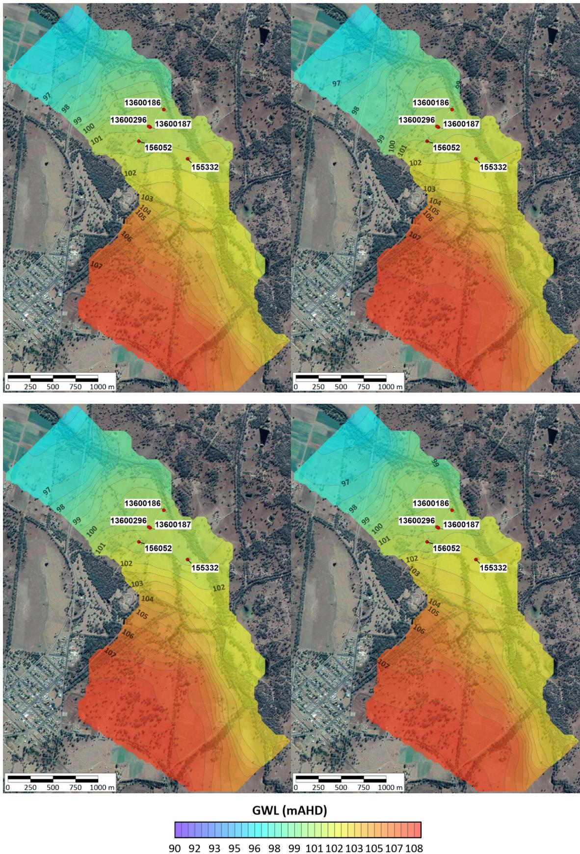
Figure 6.3. Contours of model-calculated groundwater heads for 1st February, 2011 for stochastic realisations 6 (top-left), 173 (top-right), 199 (bottom left) and 213 (bottom right).
