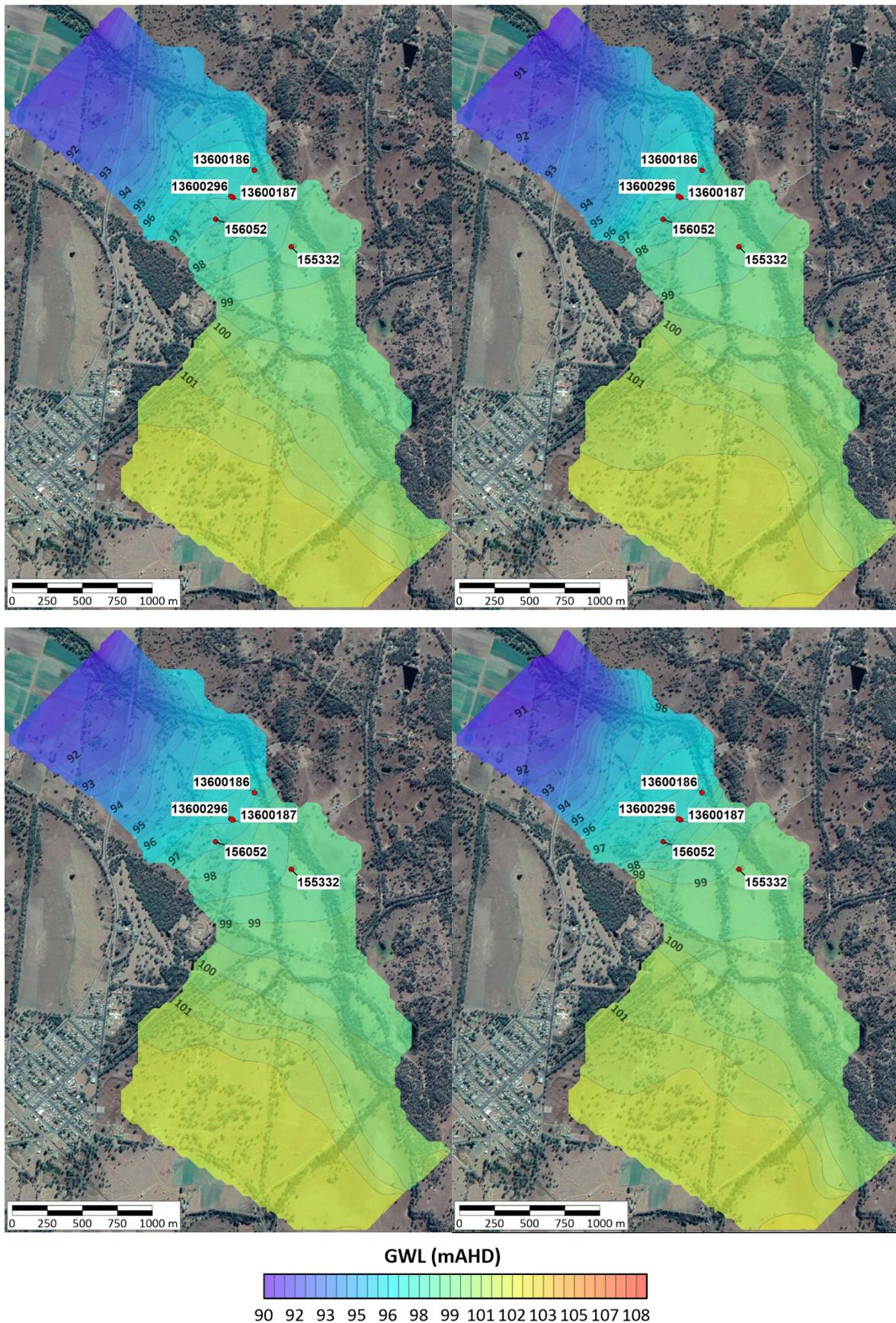
Figure 6.4. Contours of model-calculated groundwater heads for 1st November, 2006 for stochastic realisations 6 (top-left), 173 (top-right), 199 (bottom left) and 213 (bottom right).
