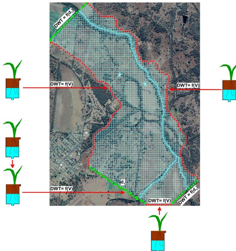
Figure 2.4a. Time-varying heads ascribed to lateral boundary conditions of the Biggenden groundwater model are calculated using four dedicated LUMPREM models for depth-to-water (DWT), one of which is actually a dual LUMPREM model. The boundary conditions on the eastern, western and southern sides of the model are GHBs. Conditions on the northern, south-eastern and south-western alluvial boundaries are represented by CHDs.
