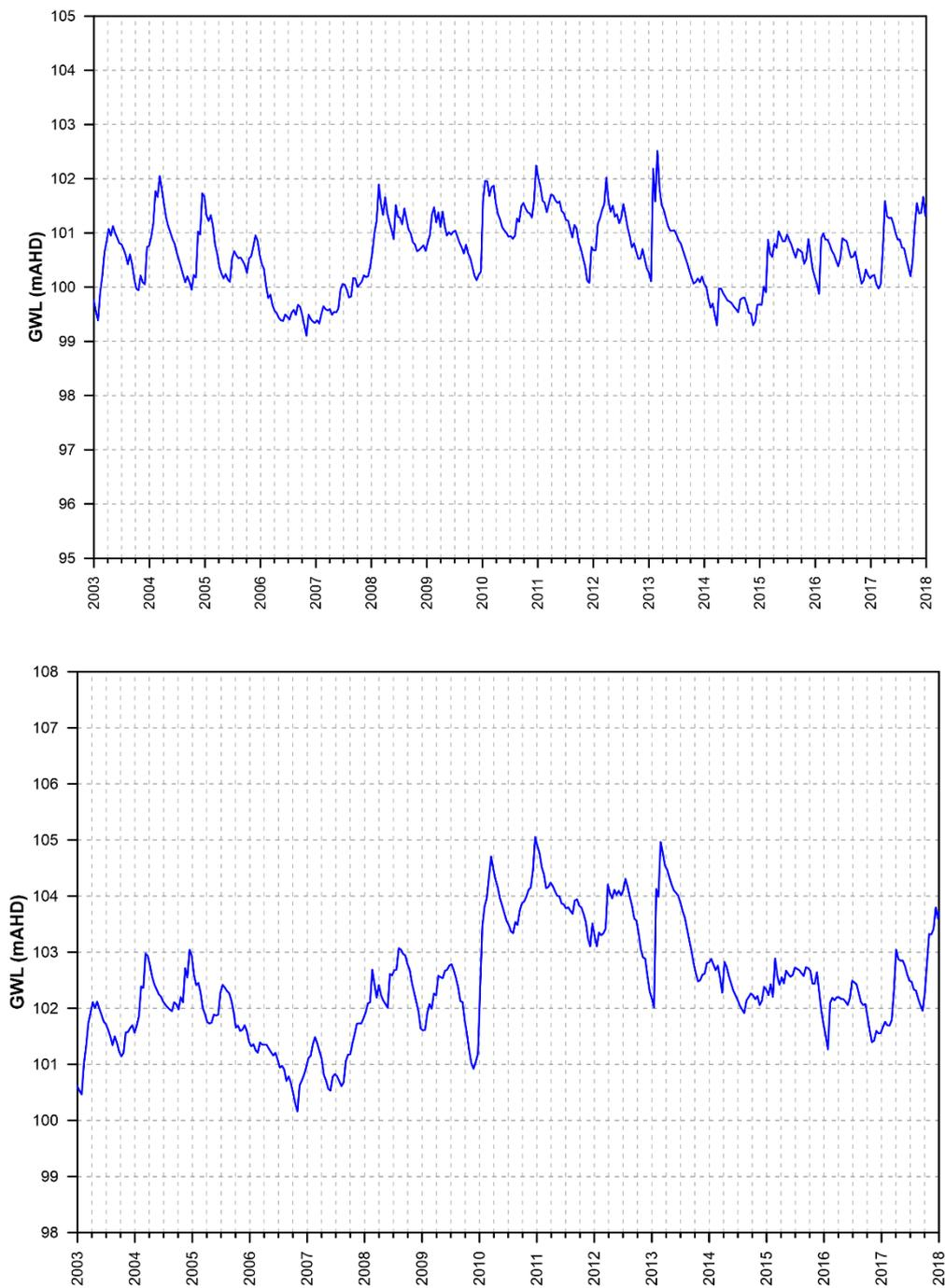
**Figure 5.5. Heads at points about half way along the eastern (top) and western (bottom) boundaries of the Biggenden groundwater model domain.**
