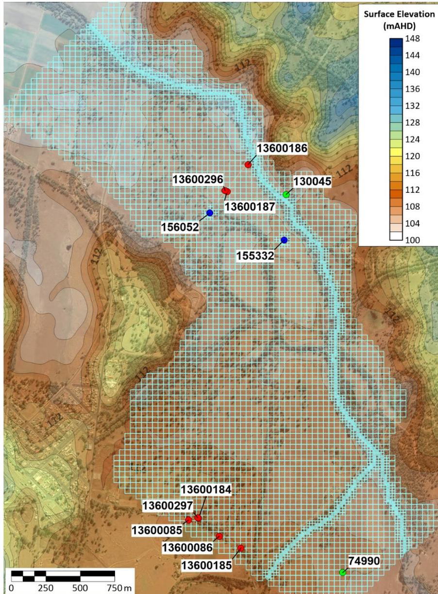
Figure 2.2. The domain of the Biggenden groundwater model; topography is also shown.
