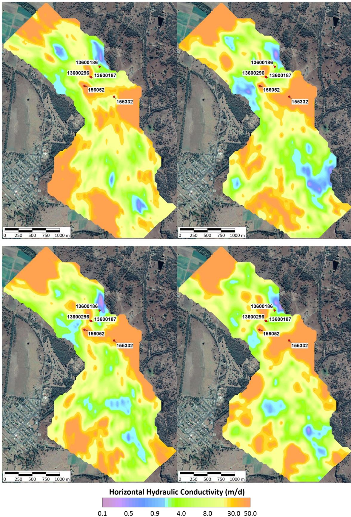
Figure 6.5. Hydraulic conductivity (i.e. Kh) parameter fields for stochastic realisations 6 (top-left), 173 (top-right), 199 (bottom left) and 213 (bottom right).
