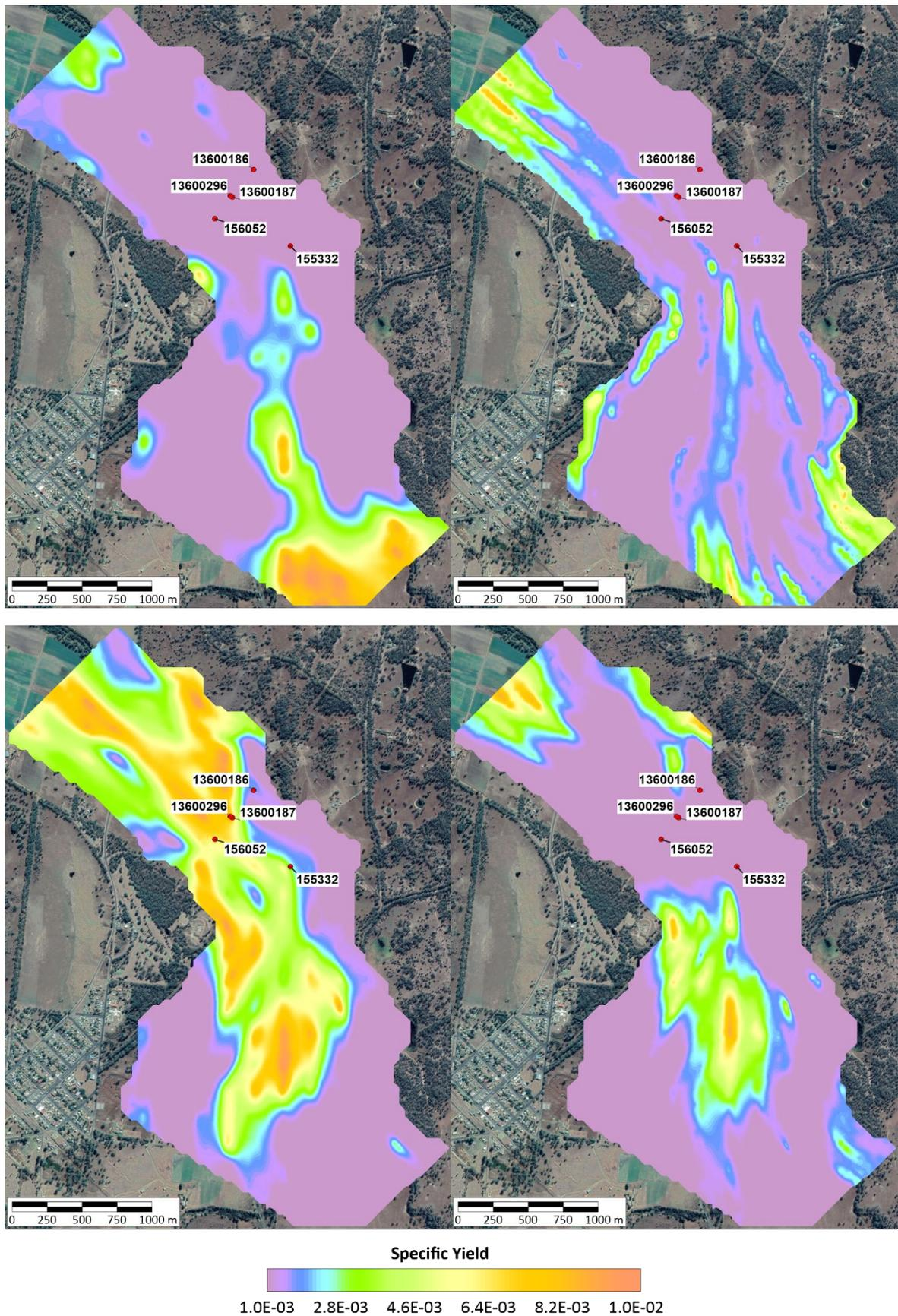
Figure 6.6. Specific yield (i.e. Sy) parameter fields for stochastic realisations 6 (top-left), 173 (top-right), 199 (bottom left) and 213 (bottom right).
