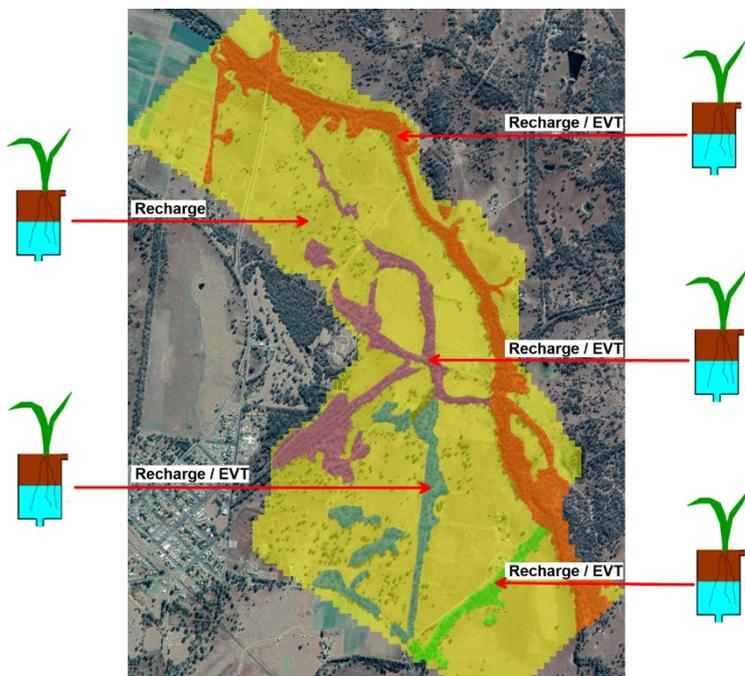
Figure 2.4b Recharge is supplied to the MODFLOW 6 RCH package of the Biggenden groundwater model using five incidences of LUMPREM. Four of these LUMPREM incidences also provide maximum EVT rate to the MODFLOW 6 EVT package.
