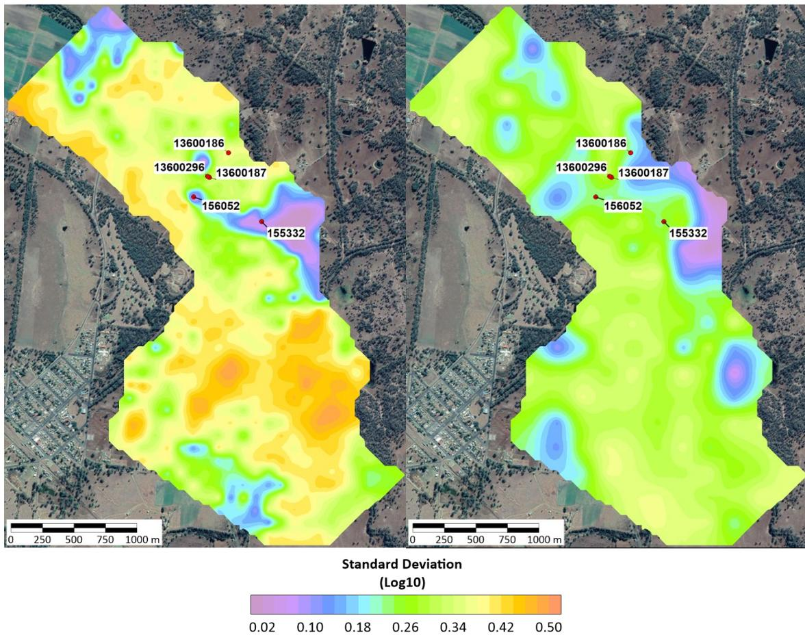
Figure 6.7. Spatial distribution of the posterior standard deviation of the best 250 parameter fields of  $\log(Kh)$  (left) and  $\log(Sy)$  (right).
