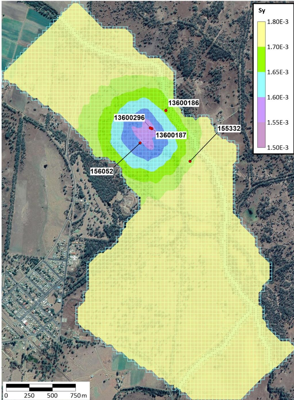
**Figure 5.7. Calibrated specific yield (i.e.  $S_y$ ) parameter field.**
