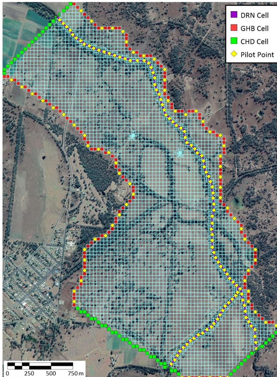
Figure 2.6. Pilot points used for parameterisation of GHB and DRN boundary conductances.
