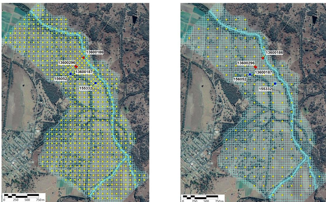
Figure 2.5a. (left) Pilot points used for parameterisation of hydraulic conductivity (Kh).
