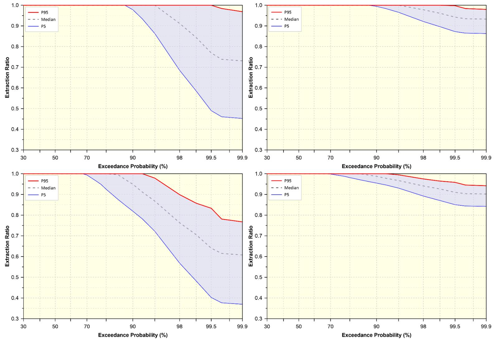
Figure 7.2. Extraction ratio exceedance probability based on the uncertainty of future weather for RN155332 at 80ML/yr demand (top left), total bore field at 80ML/yr demand (top right), RN155332 at 125ML/yr demand (bottom left) and total bore field at 125ML/yr demand (bottom right).
