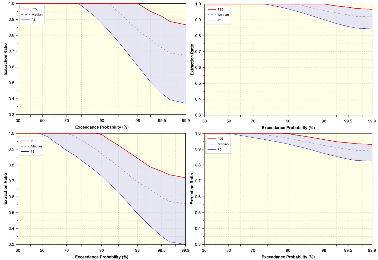
Figure 7.3. Extraction ratio exceedance probability based on both parameter and weather uncertainty for RN155332 at 80ML/yr demand (top left), total bore field at 80ML/yr demand (top right), RN155332 at 125ML/yr demand (bottom left) and total bore field at 125ML/yr demand (bottom right).
