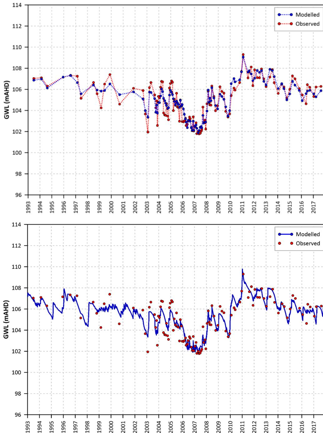
**Figure 2.3** Measured and model-calculated water levels in bore RN13600185. The latter are displayed for LUMPREM (a) at times of water level observations (top) and (b) at regular, fortnightly intervals (bottom).
