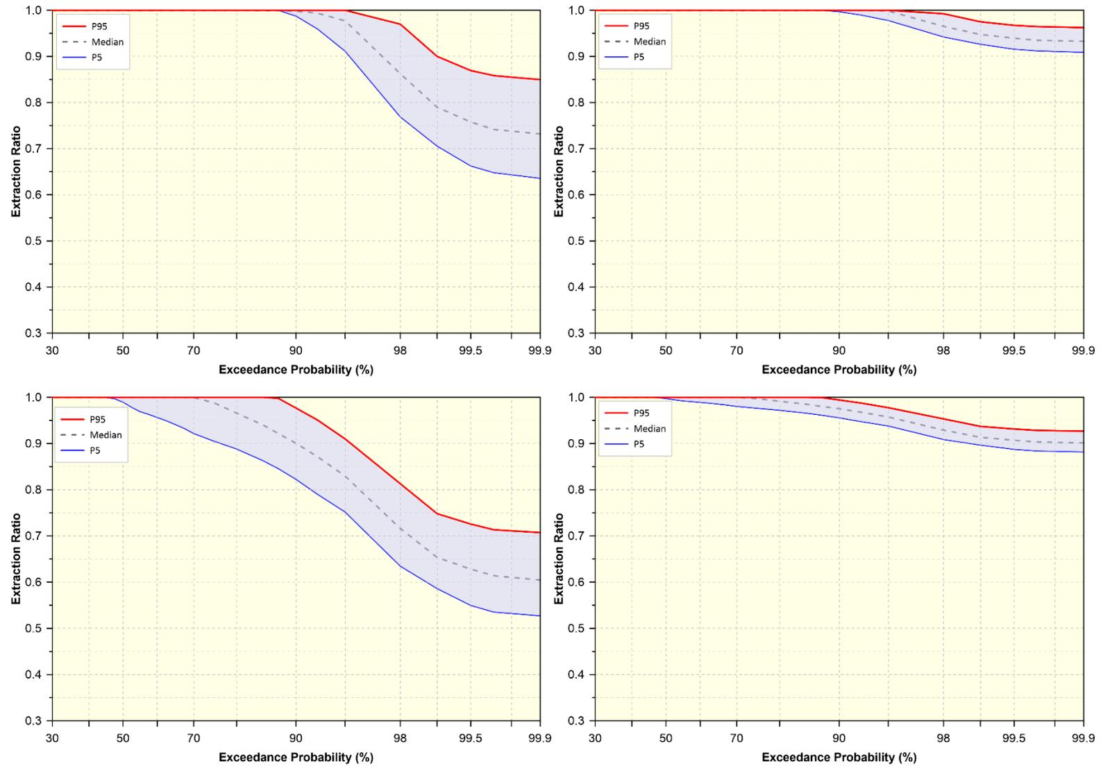
Figure 7.1. Extraction ratio exceedance probability based on parameter uncertainty for RN155332 at 80ML/yr demand (top left), total bore field at 80ML/yr demand (top right), RN155332 at 125ML/yr demand (bottom left) and total bore field at 125ML/yr demand (bottom right).
