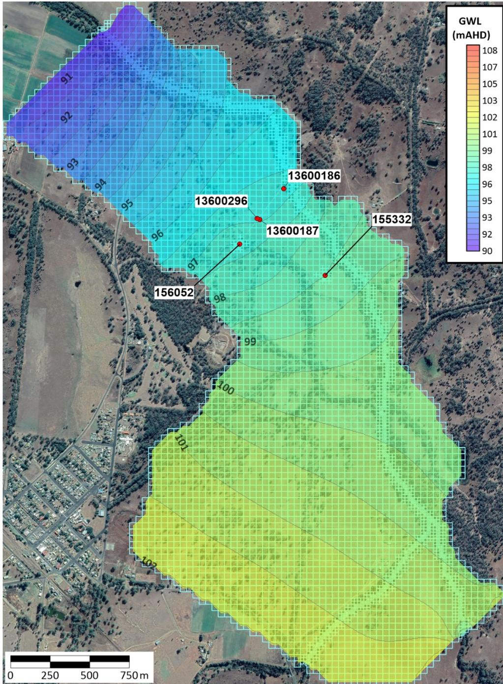
Figure 5.4. Contours of model-calculated groundwater heads for 1st November, 2006.
