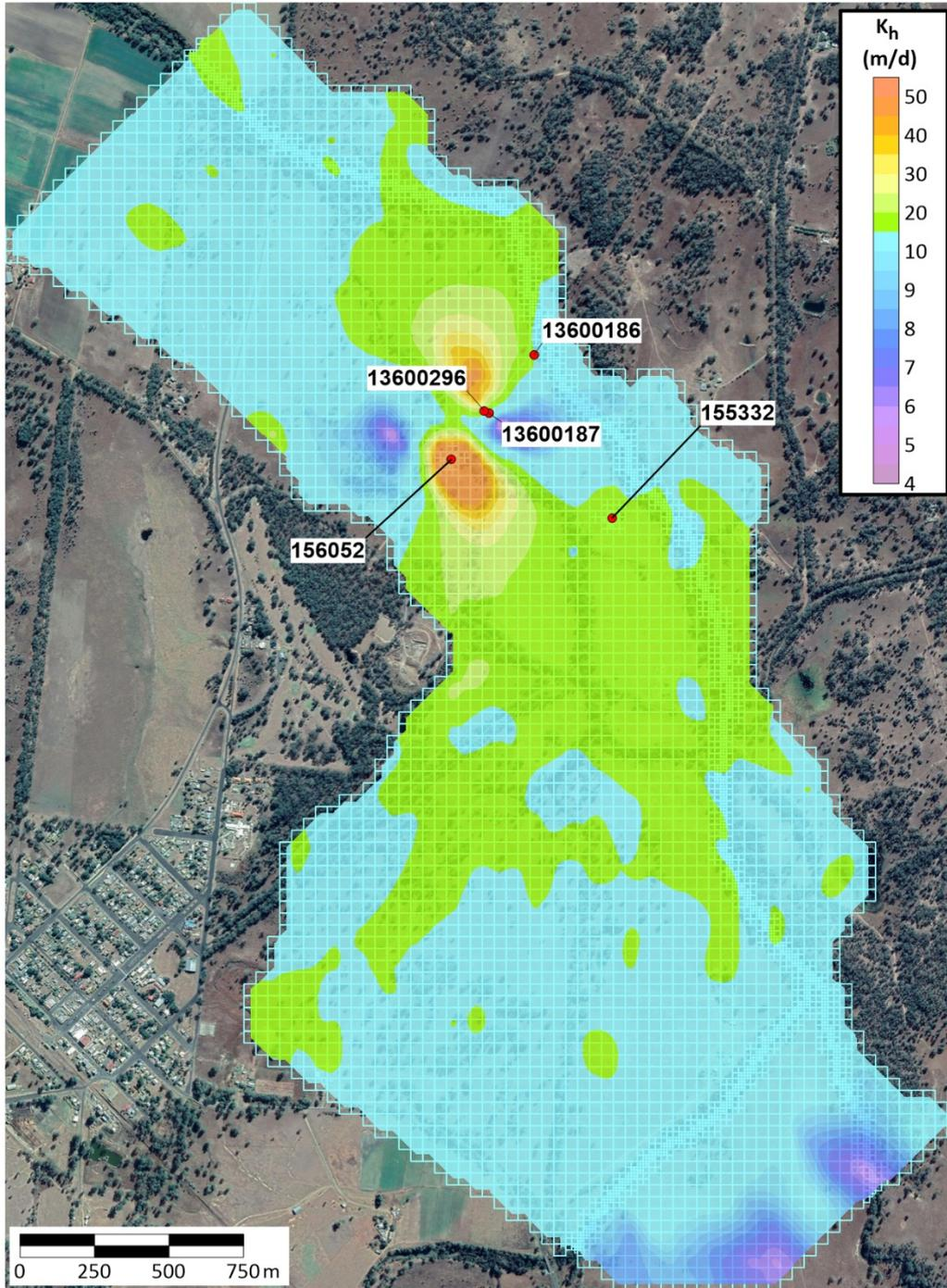
Figure 5.6. Calibrated hydraulic conductivity (i.e.  $K_h$ ) parameter field.
