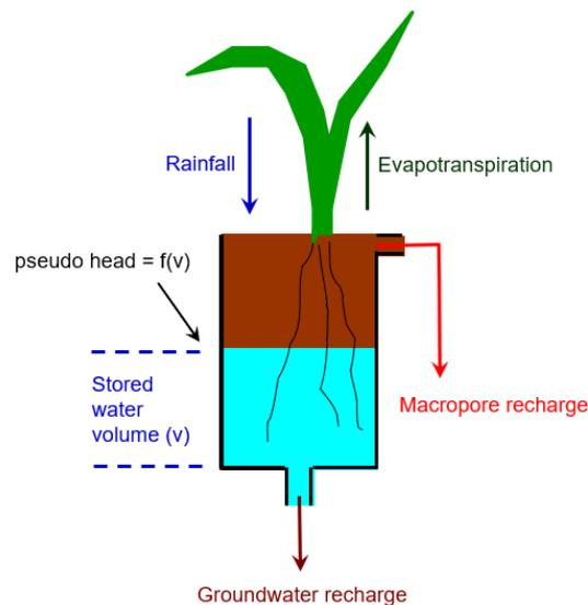
**Figure 2.1. Schematic of the LUMPREM recharge model.**
