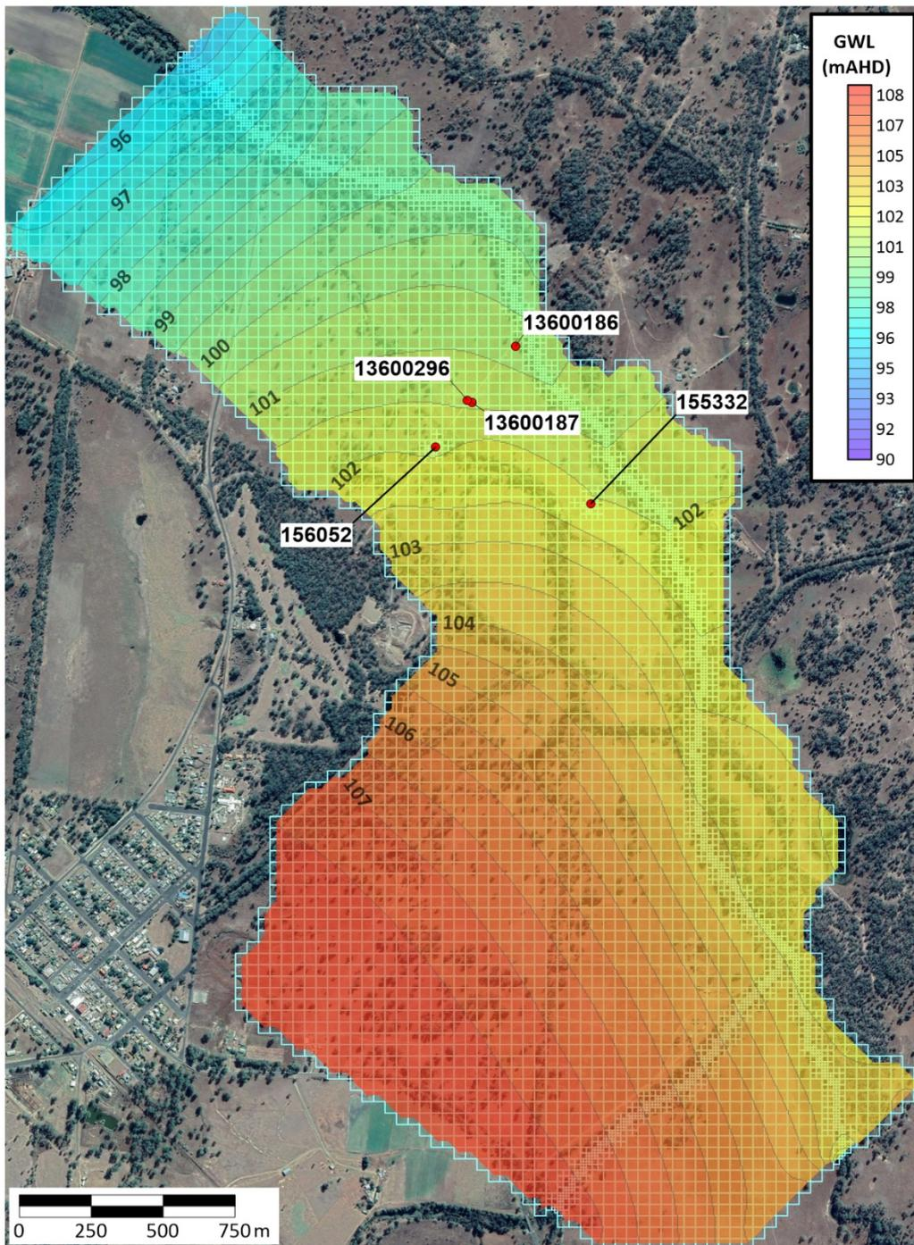
Figure 5.3. Contours of model-calculated groundwater heads for 1st February, 2011.
